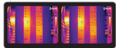
Original IR Image on the Left and with MSX ™ Enhancement on the Right image
